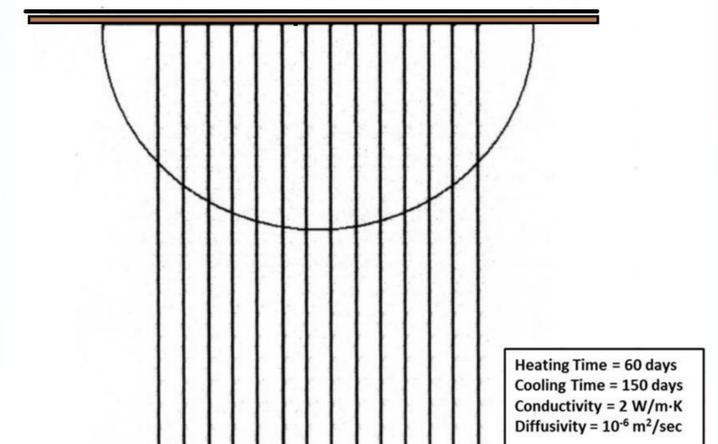
Figure 4: Underground thermal storage simulation
