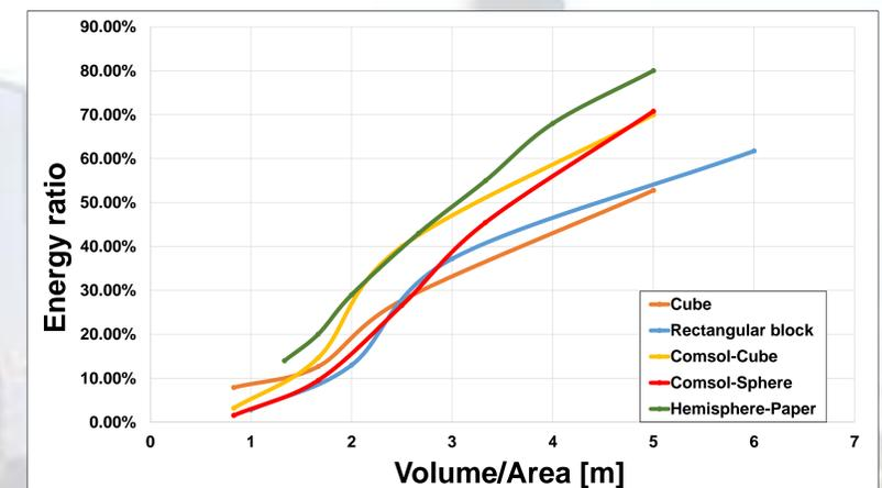
Figure 5: Underground heat/energy retention ratio
