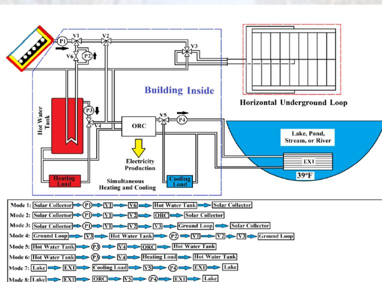
Figure 3: HVAC System with Seasonal Storage and Electricity Generation
