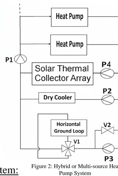
Figure 2: Hybrid or Multi-source Heat Pump System
