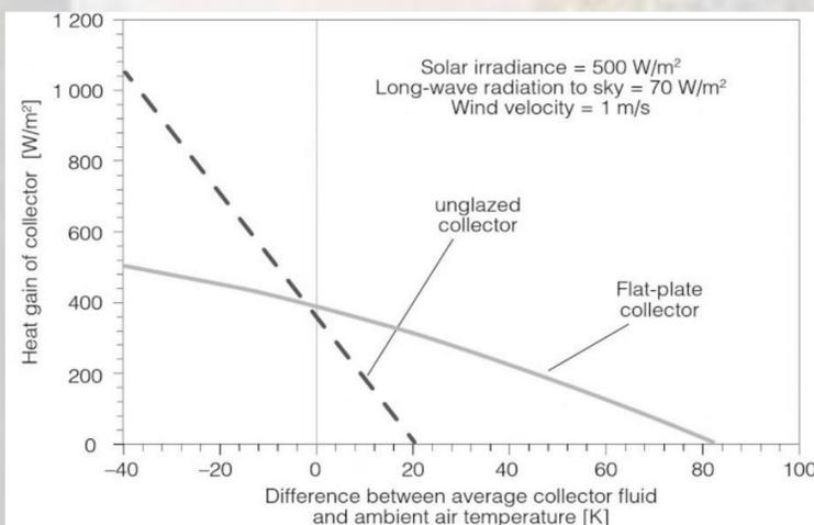
Fig. 1: Solar Thermal Collector Performance (Hadorn et al., 2015)
